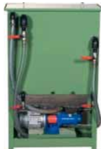
Primary chamber (Gravity settlement).
